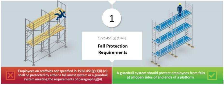
To ensure adequate protection, install guardrails along all open sides and ends before releasing the scaffold for use by employees, other than the erection and dismantling crews.
