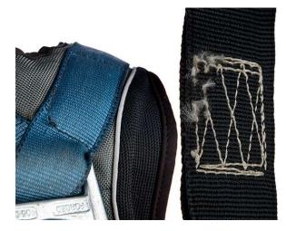
If defects are found the harness should be destroyed and disposed of to prevent use.
