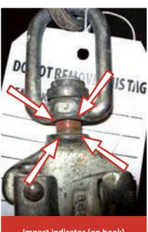
Impact indicator (on hook) ruptured, showing unit was involved in a fall. (See red indicator line)
