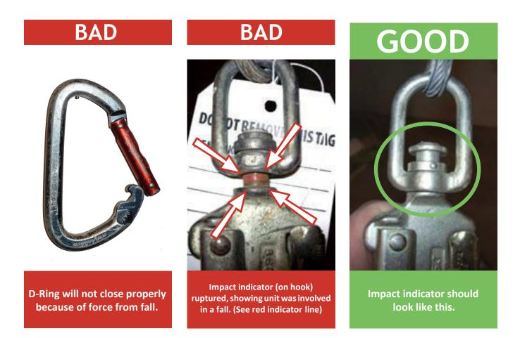
Once involved in a fall, these units are designed to tear the inside gears to slow down a fall. They will not work properly after they have been involved in a fall. Inspect all fall protection equipment before each use and tag it out of service if you have any concerns on its condition.
